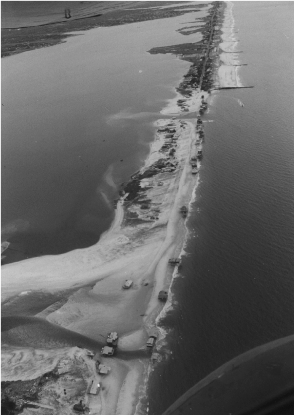
Figure 2: View to the east of the two barrier island breaches caused by the diminished sand supply and the December 11-14 Nor'Easter. Littoral drift is from east (top) to west (bottom). Photograph by Dan Covello & Aram Terchunian.
